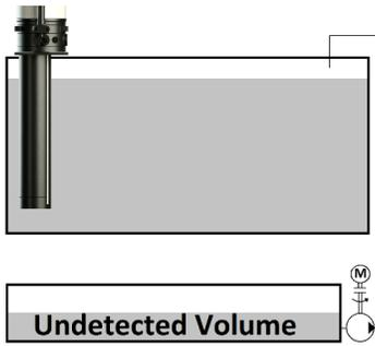
The volume to enter into the Device is either the Coolant inside the tank, but not yet detected by the Device, and/or the Coolant in a separate tank that can never be measured by the Device.
