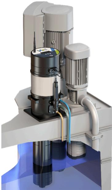
Always install the Device in the main Coolant Tank of your Process. This is where you typically organize the **periodic refills**. In most cases, this is near the pumps that supply the clean Coolant to the Machine. It's important that Will-Fill can detect the consumption of Coolant by level fluctuations inside the Coolant tank. If this is not possible consult your local distributor or Will-Fill.
