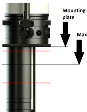
The maximum value is measured in centimeters from the base plate down to the Emulsion level.
