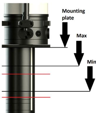
The minimum value is measured in centimeters from the base plate down to the Emulsion level.
