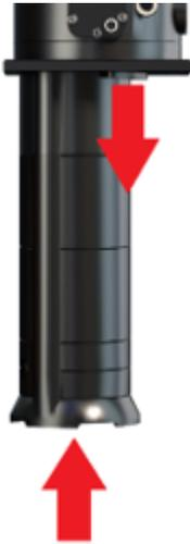
For good operation and flow of the Coolant, it is important to keep the inlet (arrow facing upwards) and outlet (arrow facing downwards) clear at all times. Notice that the outlet is ends slightly lower than the rectangular base plate. The outlet should be inside the mounting hole of the Coolant. In this way, there can be a perfect stream of emulsion in and around the Device.
