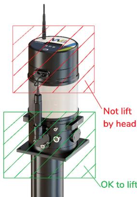
For lifting the Device, preferably use the handles on either side or the rectangular base plate if more convenient.
