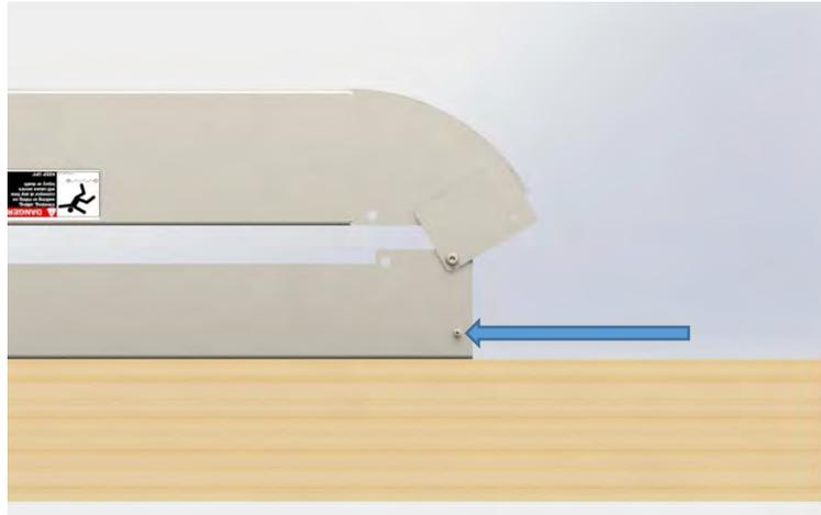
**Figure 1.2 – Screw to be Removed (Both Sides)**
